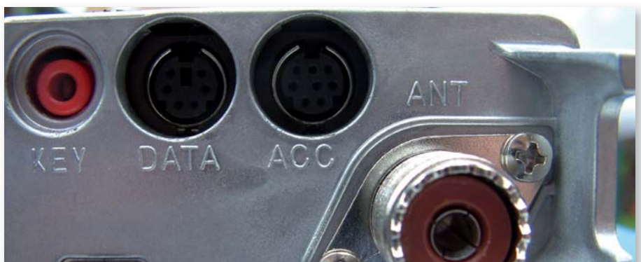
Fig. 5: The SO239 r.f. connector (bottom right) and the red 3.5mm jack socket for Morse keys (top left) on the rear panel of the Yaseu FT-817ND.
