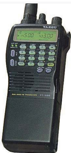
The Yaesu FT-530 is one of a few hand-helds that uses a backup lithium battery in a slot-in compartment.
