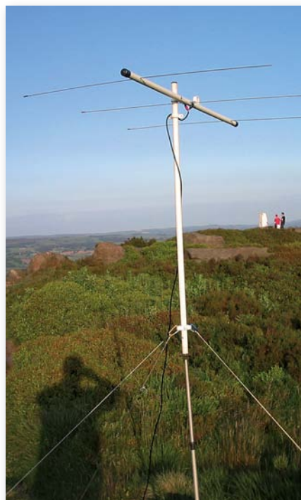
A 2-element SOTA Beam on The Cloud SP-015.
