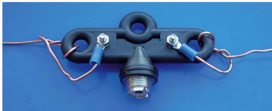
Fig. 2: A useful dipole centre with a PL-259 socket.
