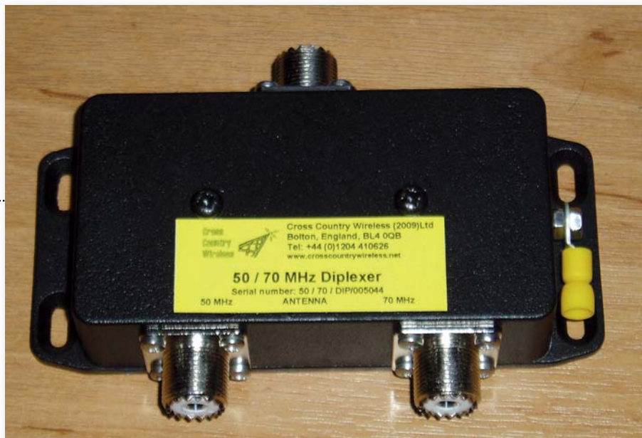
Fig. 2: Cross Country Wireless 50/70MHz Diplexer.
