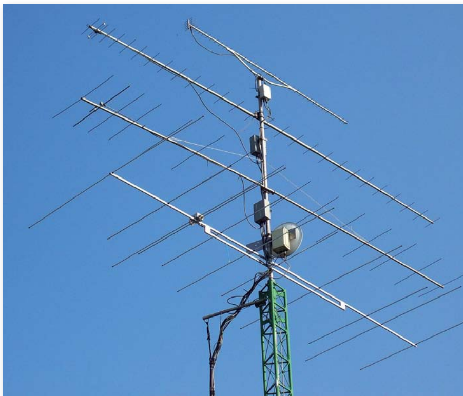
Fig. 1: The 50/70MHz dual-band Yagi (with other v.h.f., u.h.f. antennas above) at the QTH of Uffe Lindhardt PA5DD.
