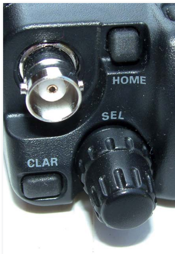
Fig. 6: The left-hand side of the Yaesu FT-817ND front panel showing the main SEL rotary control.
