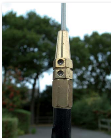
Fig. 4: Adjustment screws on a mobile whip antenna. When loosened the top section of the whip antenna can be adjusted to obtain the best v.s.w.r. readings possible.
