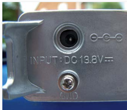
Fig. 1: The coaxial external d.c. power socket on the rear panel of the Yaesu FT-817ND, clearly show the correct polarity.
